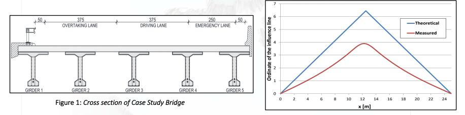
Figure 2: Difference between theoretical and SHM measured influence line
