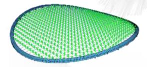
FEM model for anlyzed tendon large span structure
