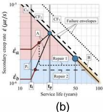
Figure: (a) shows the probability of failure evolution considering the repairs and the different pathologies modeled. (b) is the same information of the Figure (a) but in the secondary creep rate space, which is the main indicator of the model.
