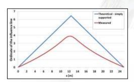
Figure 1: Difference between measured and theoretical influence line
