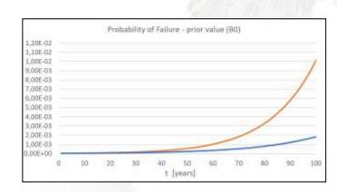
Figure 1: Probability of failure progression trough service life
