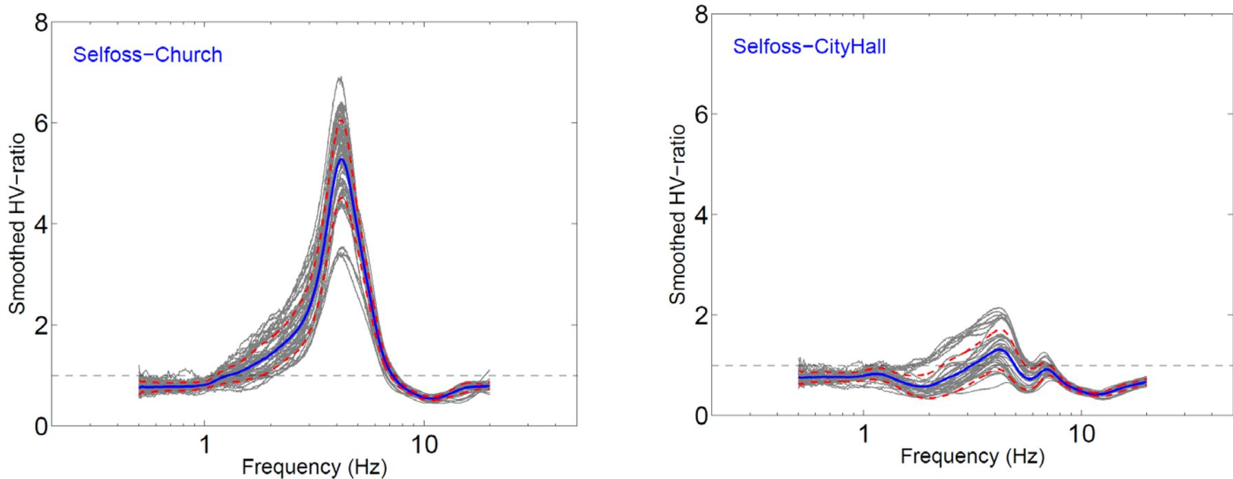
Mean Horizontal to Vertical Spectral Ratio (HVSR)  $\pm$  one standard deviation from ambient noise measurements. The grey lines show 20-min ambient noise windows used to derive the mean HVSR (blue line) and standard deviation (red dashed line). The instruments used were a Lennartz LE-3D/5s seismometer and a REF TEK 130-01 Broadband Seismic Recorder.
