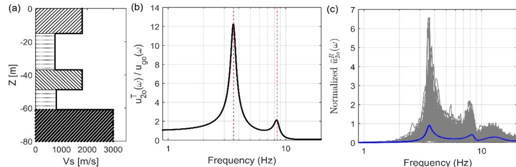
(a) Vs profile (b) The ratio of absolute displacement frequency response at the surface to the ground displacement at the bottom. (c) Relative acceleration frequency response of horizontal motion at the free-surface for the 2DOF system .
