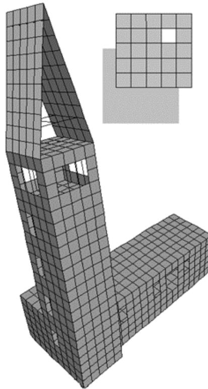
*The first mode of vibration has a frequency of 5 Hz*
