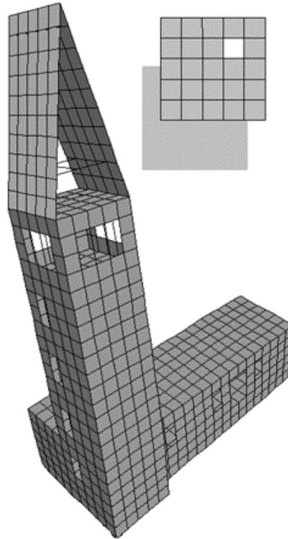
*The first mode of vibration has a frequency of 5 Hz*
