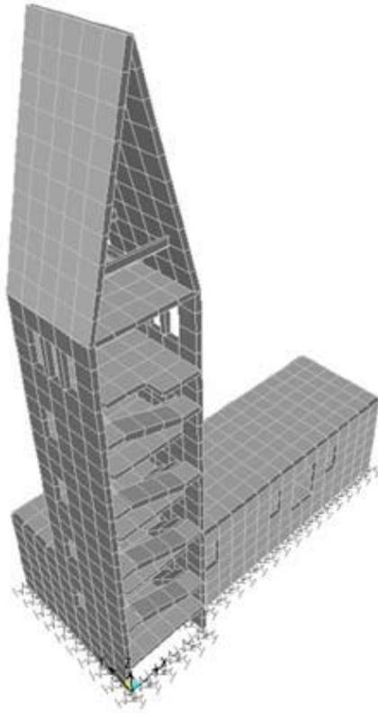
*The Finite element model with spring supports*
