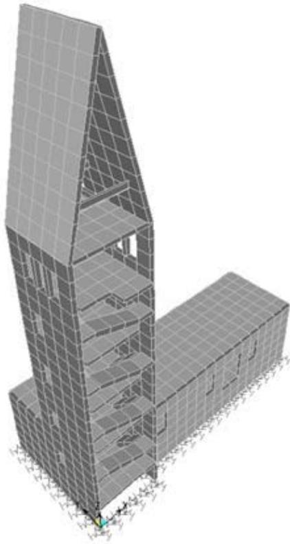
*The Finite element model with spring supports*
