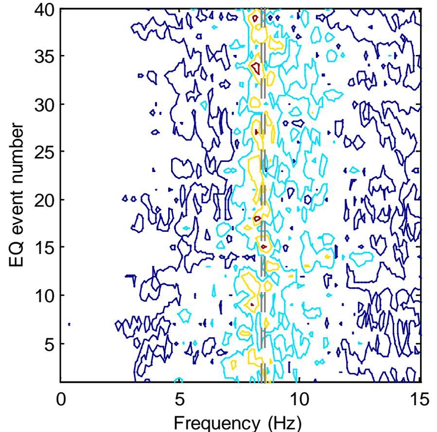
**Contour graphs of the Fourier spectrum for the 40 events analysed. (a) Vibration in the NNE-SSW dir. & (b) Vibration in the ESE-WNW direction. Double dotted lines point out the slight drift in natural frequency of each mode of vibration throughout the observation period.**
