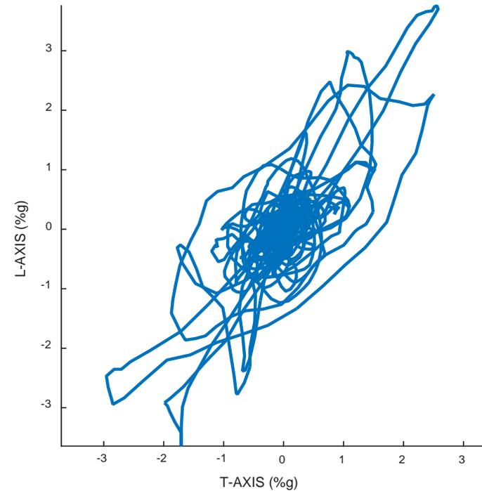
*A plot of the two horizontal acceleration components recorded in an aftershock*
