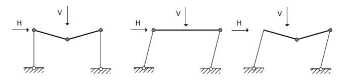
$F_i$  = event 'occurrence of i-th failure mode'  $f_j$  = event 'local failure of j-th member/cross section'
