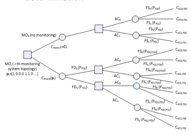
AC = actions resulting from failure detection (e.g. vehicle load restriction or bridge closure)
