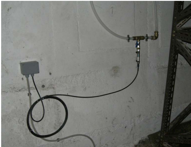
Measurement of vertical displacements (9 sections)
