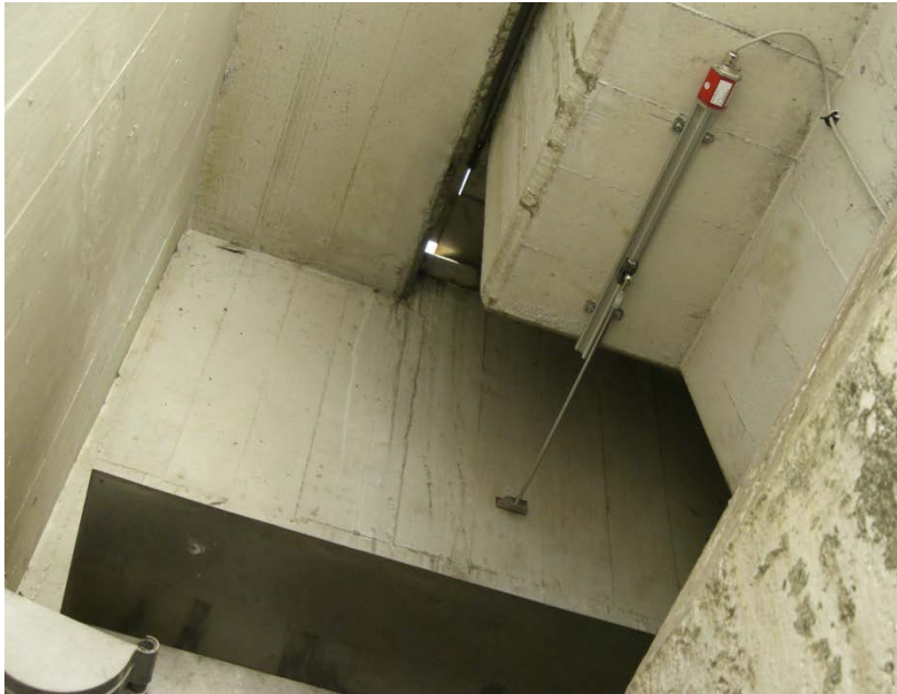
Measurement of displacements at expansion joints
