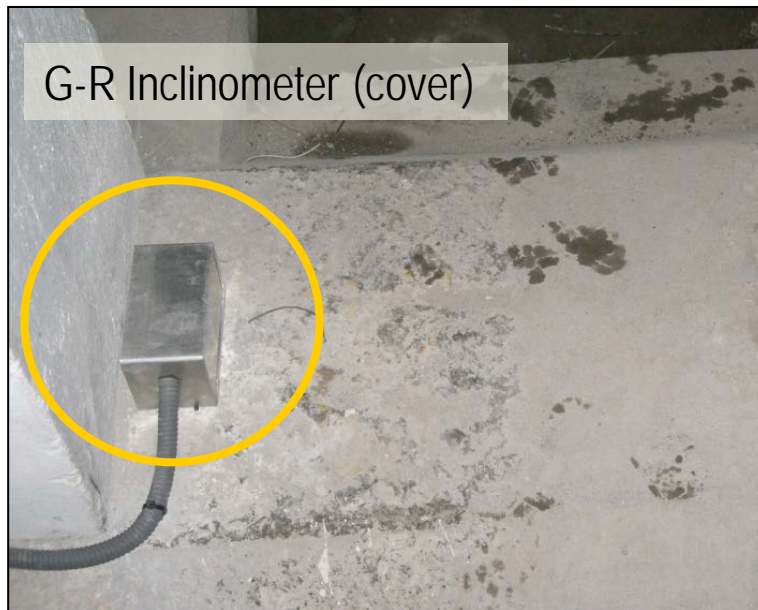
Measurement of rotations (Biaxial)
