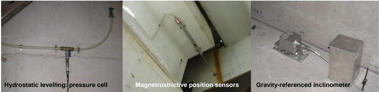
Figure 5: Sensors installed in the SHM system upgrade
