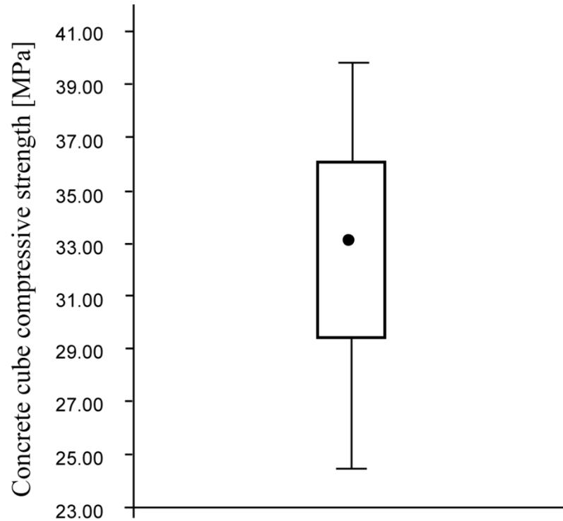
Tukey Box plot of the concrete compressive strength data
