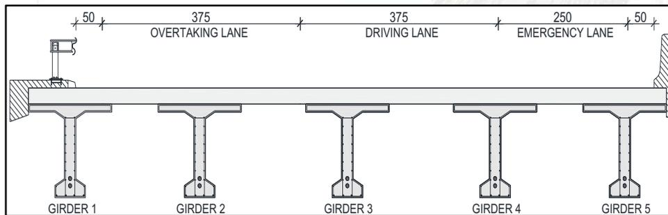
Figure 1: Cross section of Case Study Bridge
