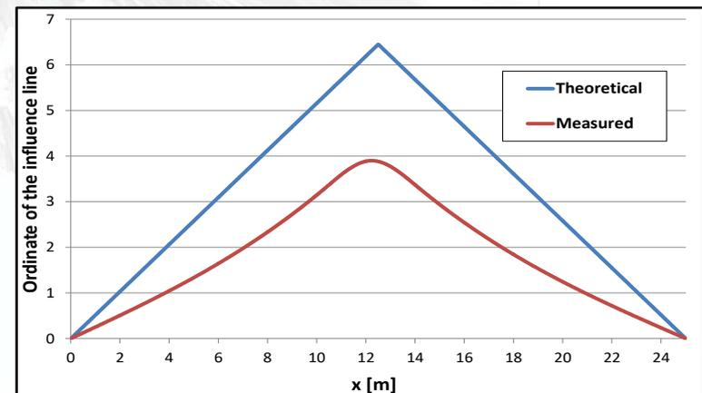
Figure 2: Difference between theoretical and SHM measured influence line
