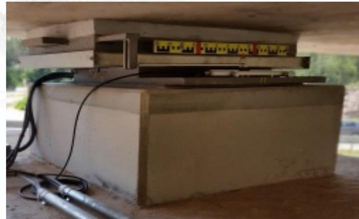
Instrumented bearing (source: BASt)
