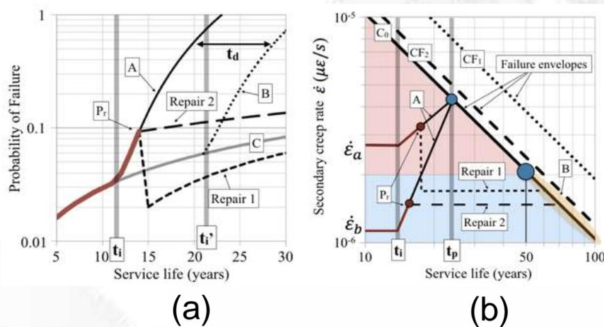
Figure: (a) shows the probability of failure evolution considering the repairs and the different pathologies modeled. (b) is the same information of the Figure (a) but in the secondary creep rate space, which is the main indicator of the model.
