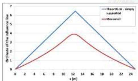
Figure 1: Difference between measured and theoretical influence line
