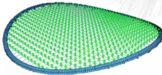
FEM model for analyzed tendon large span structure
