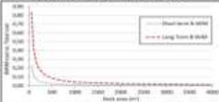
Figure 4: Ratio of SHM costs and total bridge value depending on the bridge deck area
