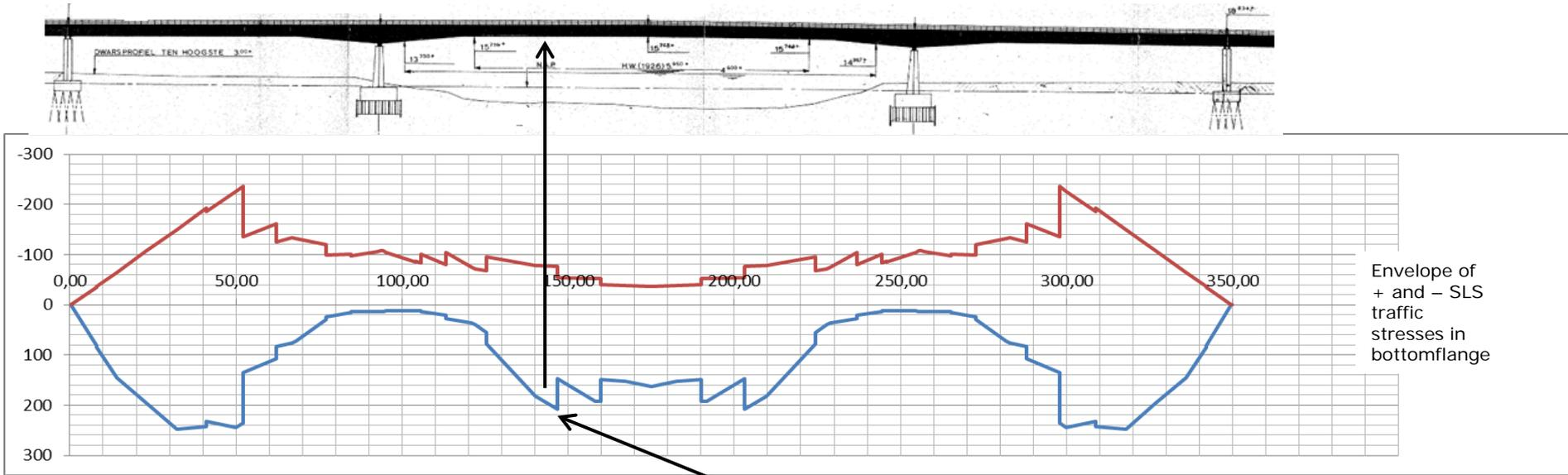
Main span max traffic stresses in bottom flange:
