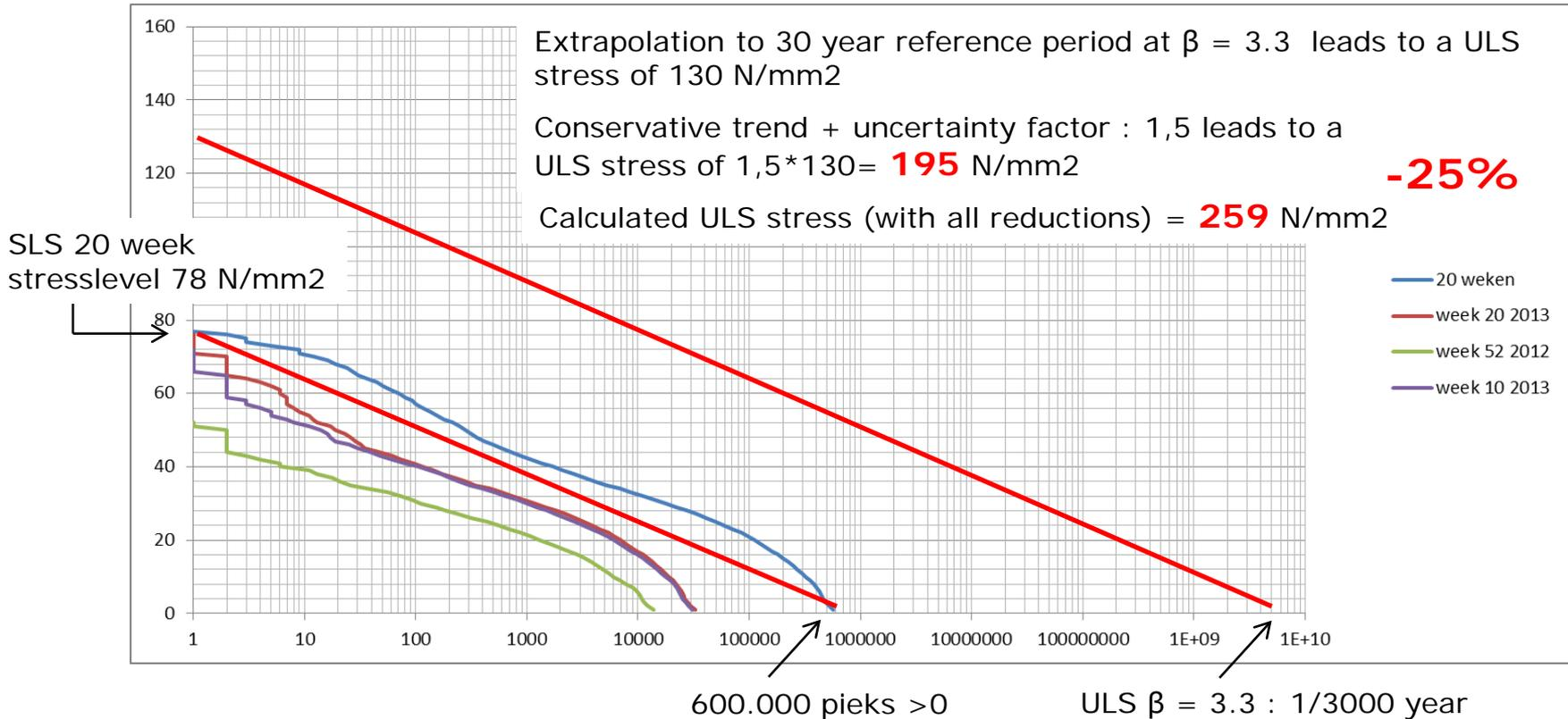
Cumulative exceedence line main span max SLS tension stress in bottom flange
