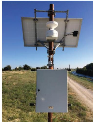
Standalone system with photovoltaic cells
