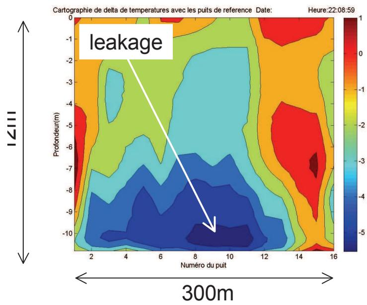
Real time monitoring of the leakage
