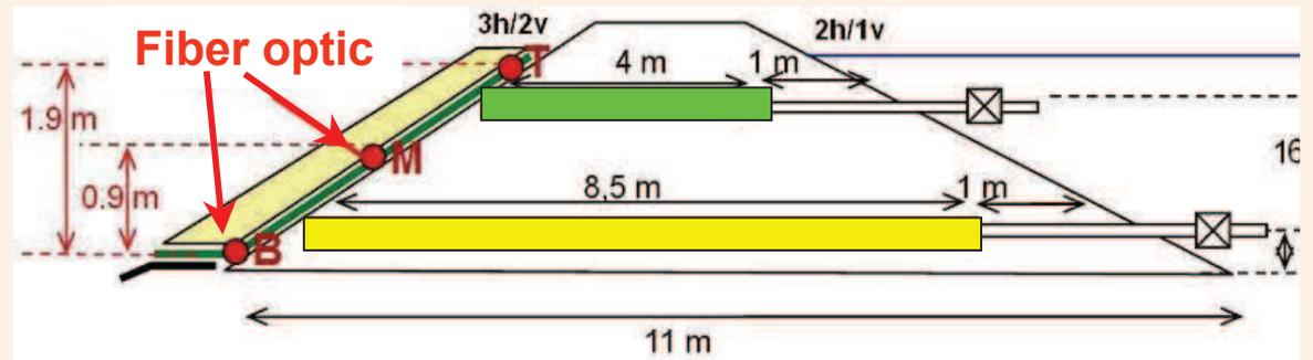
The leakage is detected by the reduction of the air temperature diffusion time
