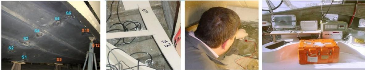
Hull pressures, strain and motion - 2004
