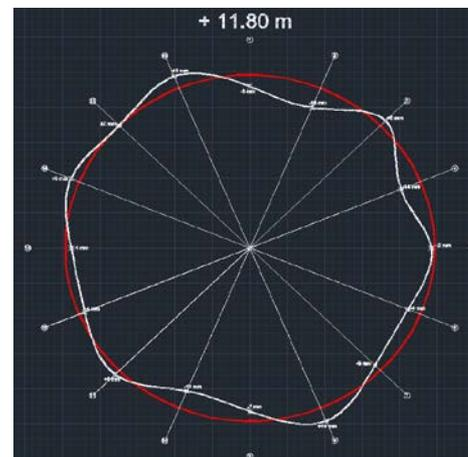
**Real geometry** measured on the fully filled tank with geodetic method
