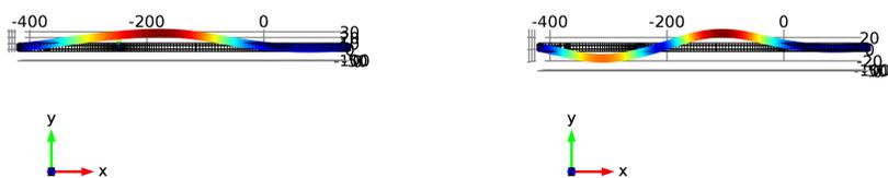
Figure 3. Mode shapes predicted by FE model
