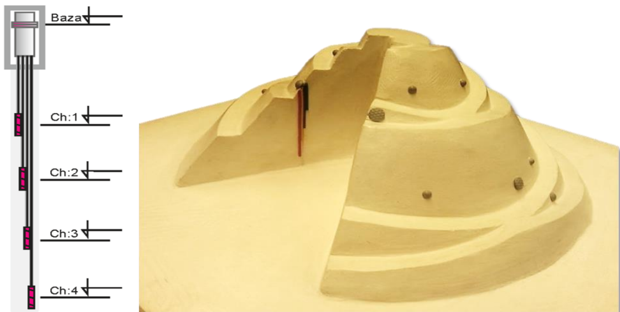
Figure 6. Details of vertical displacement measurements.
