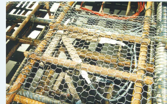
Embedded strain gages
